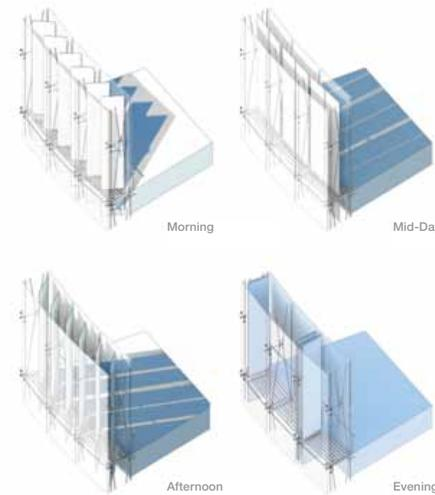
**Above** Computer-controlled louvers track sunlight throughout the day, optimizing the amount of light entering the building. **Above right** Prestressed Vierendeel trusses provide the atrium's lateral support. **Facing** In warm weather, the building's exhaust air is drawn through custom grating at each floor to a rooftop vent. **Opening spread** The climate wall and atrium give a new face to the hospital's cutting-edge facilities.
