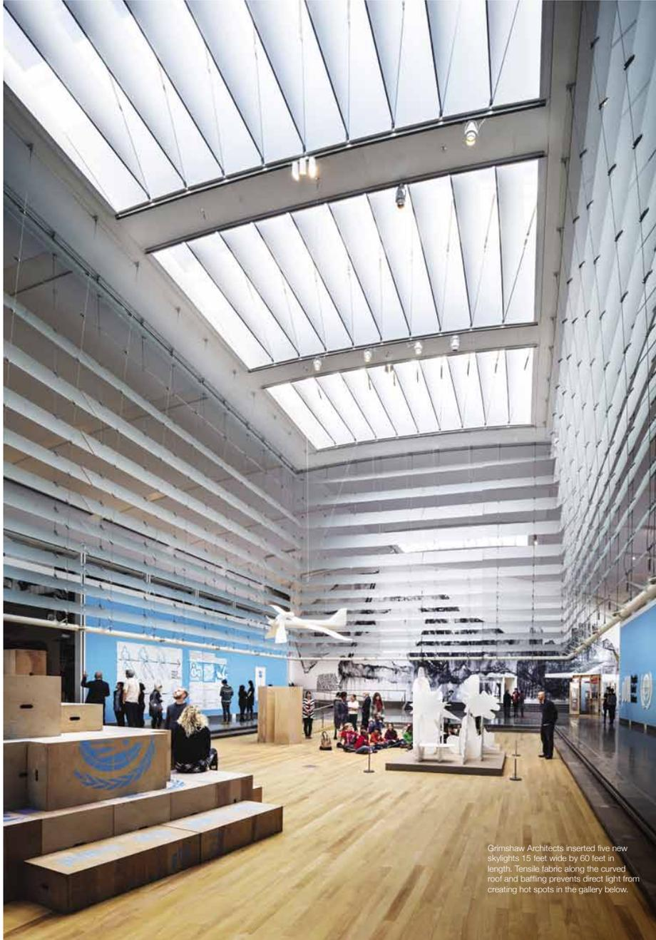
Grimshaw Architects inserted five new skylights 15 feet wide by 60 feet in length. Tensile fabric along the curved roof and baffling prevents direct light from creating hot spots in the gallery below.
