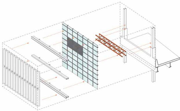
**Clockwise from left** An exploded detail of the operable curtain wall and truss structure from which it hangs. The building's west and south facades showing the curtain wall during fin installation (top) and after installation (below). The building's double-skin facade as seen from street level.
