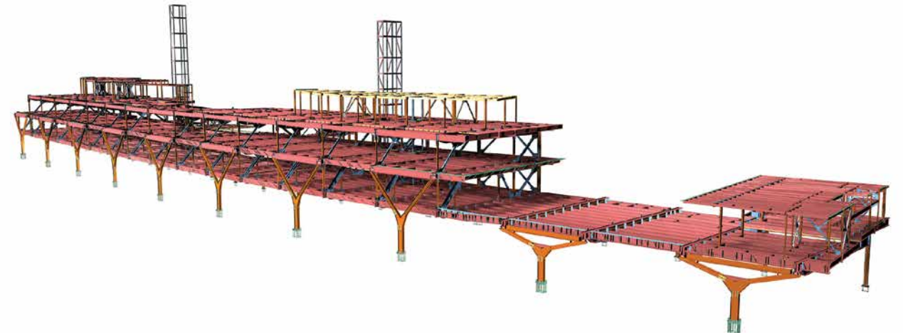
Top Supported by 10 “Y” columns overlooking FDR Drive and the East River, Rockefeller University’s new 180,000-square-foot laboratory building spans almost three and a half city blocks.
